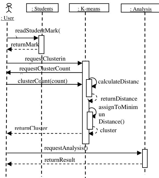
**Figure 2. Sequence diagram of the proposed system**
